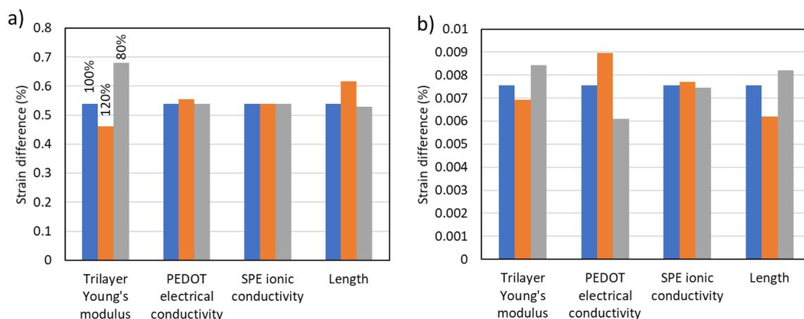
Fig. 18. Key factors affecting the actuator displacement under a square wave voltage ( $V_{pp} = 2.4$  V), a) at low frequency  $f = 0.1$  Hz, and b) at high frequency  $f = 20$  Hz. For each parameter, three columns from left to right represent for its real value (blue column), its value increased by 20% (orange column), and its value reduced by 20% (gray column).
