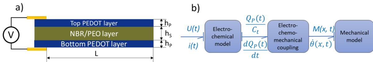
Fig. 1. a) Trilayer actuator, b) Trilayer actuator Words BG model.
