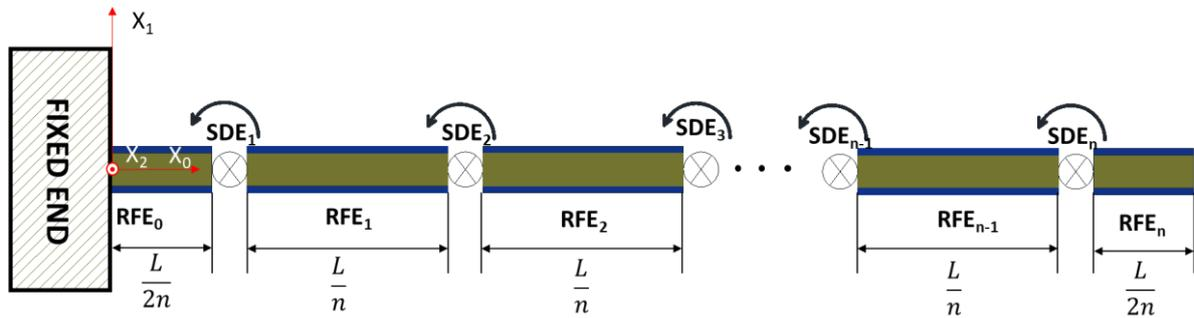
Fig. 4. Rigid Finite Element Model (RFEM) of a trilayer actuator, in which it is divided into  $(n+1)$  rigid elements: from  $RFE_0$  to  $RFE_n$ , the elements each have a mass and are linked by spring-dampers  $SDE_1$  to  $SDE_n$ , shown in their initial positions.
