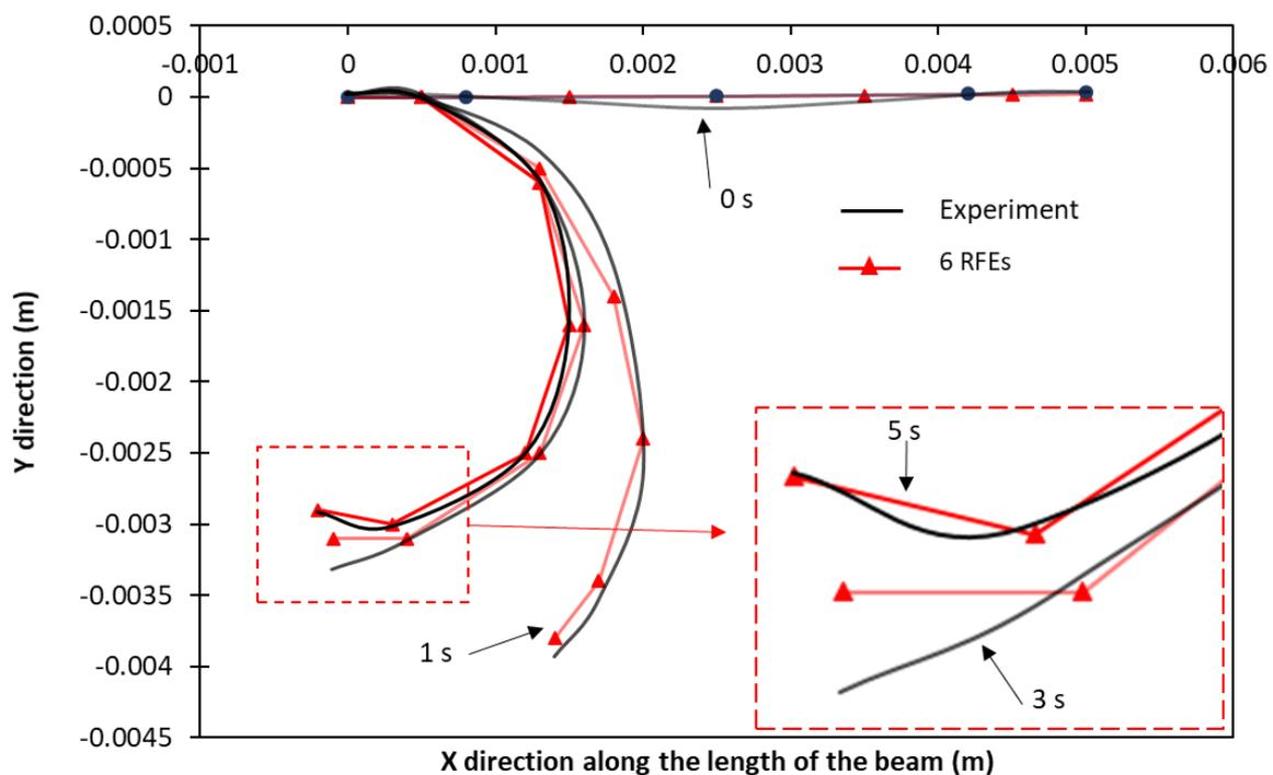
Fig. 17. Comparison between the experiment and the simulation in terms of the dynamic mechanical behavior of the beam subjected to a voltage excitation of 2.2 V<sub>pp</sub> at 0.1 Hz.
