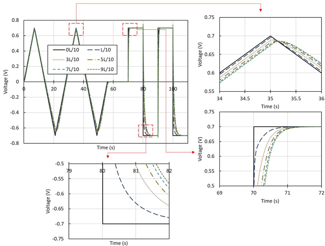
Fig. 15. Modeled voltage drops along the length of the beam due to the existence of electrical resistance of PEDOT electrodes. The legend indicates the plotting of local voltage drop as a function of distance along the trilayer from the electrical contact point, from zero (black line) to 90% of the length (fine black dash).
