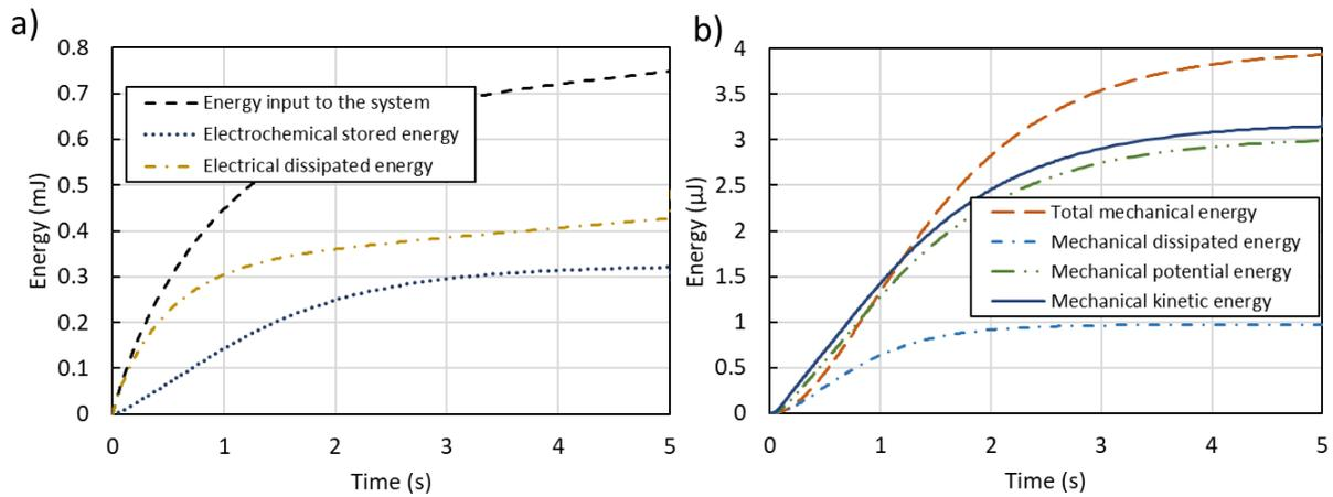
Fig. 19. Evolution of energy over half a period of applied voltage: a) The electrochemical energy, and b) The mechanical energy.
