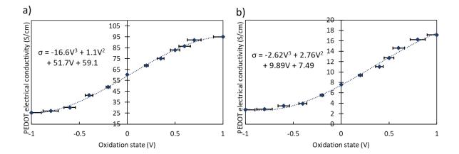
**Fig. 9.** PEDOT electrical conductivity: a) on the bottom PEDOT surface of the trilayer structure, b) on the top PEDOT surface of the trilayer structure
