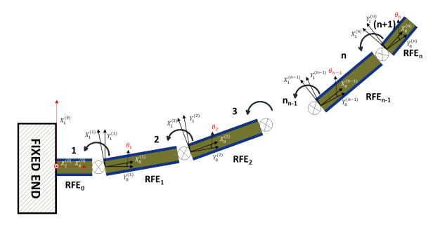
Fig. 5. Trilayer actuator in a bent state. The bending angle between the element (i-1) and the element i is  $\theta_i$ .
