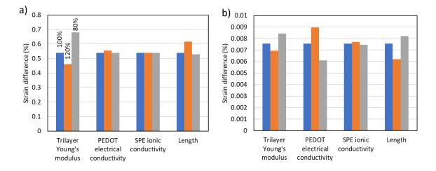
Fig. 18. Key factors affecting the actuator displacement under a square wave voltage (Vpp = 2.4 V), a) at low frequency f = 0.1 Hz, and b) at high frequency f = 20 Hz. For each parameter, three columns from left to right represent for it real value (blue column), it value increased by 20% (orange column), and it value reduced by 20% (gray column).
