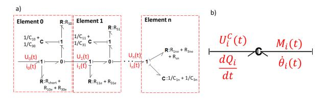
Fig. 3. a) BG representation of the electrochemical model, b) Coupling between the electrochemical subsystem and the mechanical subsystem.
