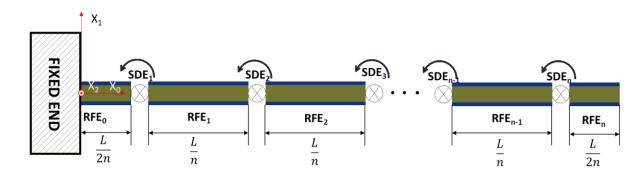
Fig. 4. Rigid Finite Element Model (RFEM) of a trilayer actuator, in which it is divided into (n+1) rigid elements: from RFE<sub>0</sub> to RFE<sub>n</sub>, the elements each have a mass and are linked by spring-dampers SDE<sub>1</sub> to SDE<sub>n</sub>, shown in their initial positions.
