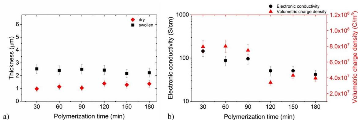
Fig. 5. Effect of EDOT VPP time on PEDOT electrode's thickness (a- $\blacksquare/\blacklozenge$ ), electronic conductivity (b- $\bullet$ ), and volumetric charge density (b- $\blacktriangle$ ). mPEG content: 10 wt%; spin coating speed/acceleration/duration of oxidant solution: 2500 rpm/1000 rpm  $\text{s}^{-1}$ /30 s; EDOT VPP temperature: 40°C.
