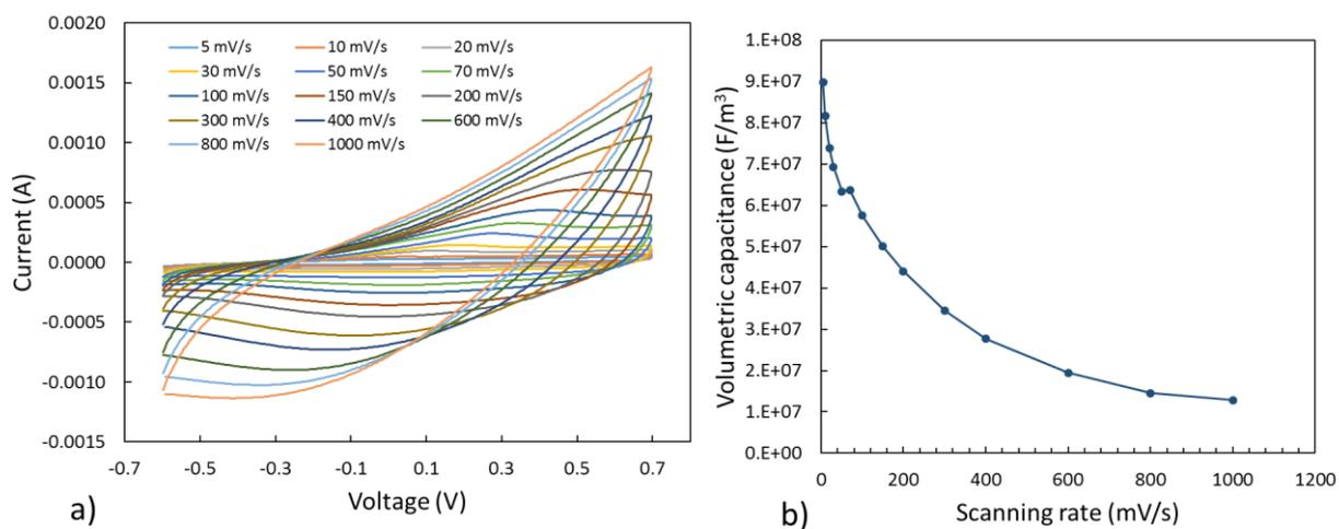
Fig. 8. a) Cyclic voltammograms of PEDOT electrodes obtained in neat EMImTFSI within a potential window of -0.6 V to +0.7 V with different scan rates: b) Volumetric capacitance of PEDOT electrodes as function of the scanning rate.
