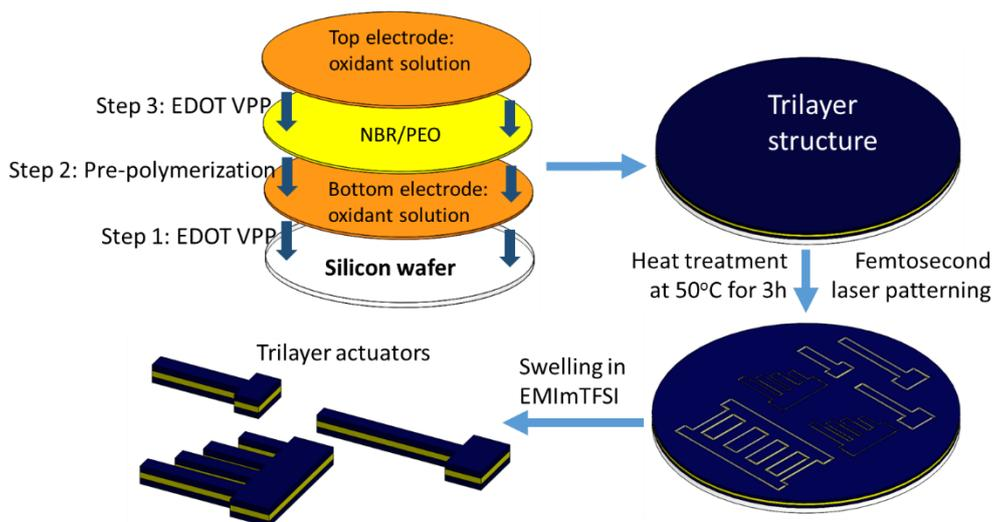
Fig. 2. Microactuator fabrication process.
