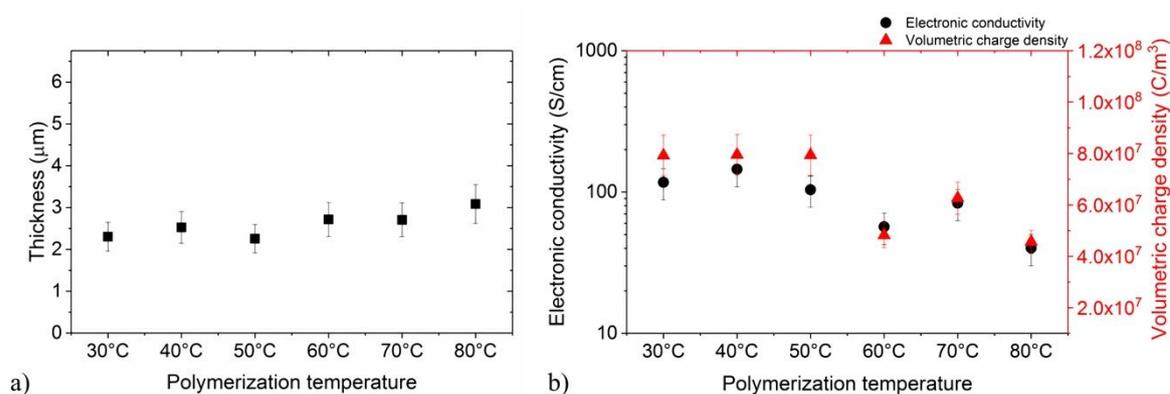
Fig. 6. Influence of EDOT VPP temperature on PEDOT electrode's thickness (a- $\blacksquare$ ), electronic conductivity (b- $\bullet$ ), and volumetric charge density (b- $\blacktriangle$ ). mPEG content: 10 wt%; spin coating speed/acceleration/duration of oxidant solution: 2500rpm/1000rpm  $\text{s}^{-1}$ /30s; EDOT VPP time: 30 min.
