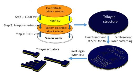
Fig. 2. Microactuator fabrication process.
