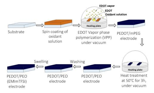
Fig. 1. Fabrication process of PEDOT electrodes.
