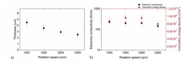
Fig. 4. Thickness (a-■), electronic conductivity (b-●) and volumetric charge density (b-▲) of PEDOT electrodes as a function of rotation speed of the spin coater. mPEG content: 10%; EDOT VPP time: 30 min; EDOT VPP temperature: 40°C. Acceleration 1000 rpm s<sup>-1</sup>, duration 30 s.
