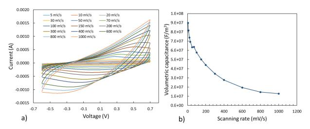
Fig. 8. a) Cyclic voltammograms of PEDOT electrodes obtained in neat EMImTFSI within a potential window of -0.6 V to +0.7 V with different scan rates: b) Volumetric capacitance of PEDOT electrodes as function of the scanning rate.
