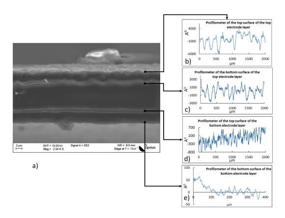
Fig. 7.a) SEM image of the trilayer cross section, profilometer surface roughness of the b) top surface of the top electrode layer, c) top surface of the SPE of a bilayer PEDOT/SPE, d) top surface of the bottom electrode layer.
