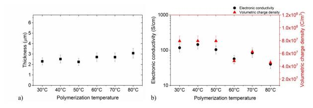
Fig. 6. Influence of EDOT VPP temperature on PEDOT electrode's thickness (a-■), electronic conductivity (b-●), and volumetric charge density (b-▲). mPEG content: 10 wt%; spin coating speed/acceleration/duration of oxidant solution: 2500rpm/1000rpm s<sup>-1</sup>/30s; EDOT VPP time: 30 min.
