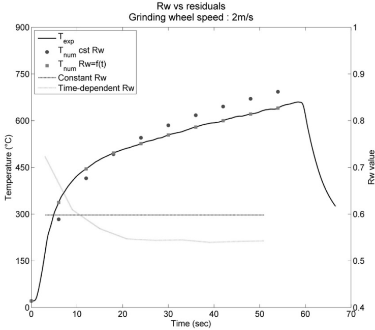
Figure 4 – Temperature and estimated R_w value for h_{eq}=7nm – Wheel 1
