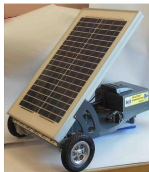
Fig 3: An autonomous rover equipped with a solar panel
