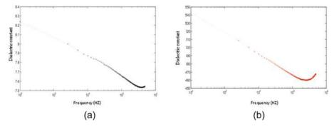
Figure 5. The variation of the dielectric constant of the PZT (a) and PU (b) according to the frequency.
