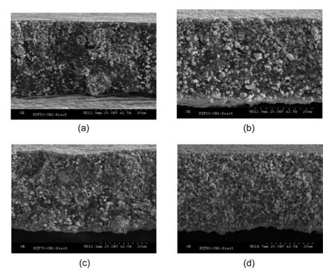
**Figure 2.** Scanning electron microscopy images of samples with different volume fraction of PZT (a): Dispersion of 50% of PZT into the matrix (b): Dispersion of 60% of PZT into the matrix (c): Dispersion of 70% of PZT into the matrix (d): Dispersion of 80% of PZT into the matrix.
