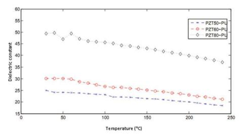
Figure 7. The variation of the dielectric constant of the PZT/PU composite according to temperature.
