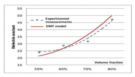
Figure 3. Concentration dependent dielectric constant of PZT/PU
