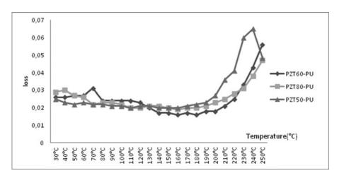
**Figure 8.** The variation of the dielectric loss of the PZT/PU composite according to temperature.
