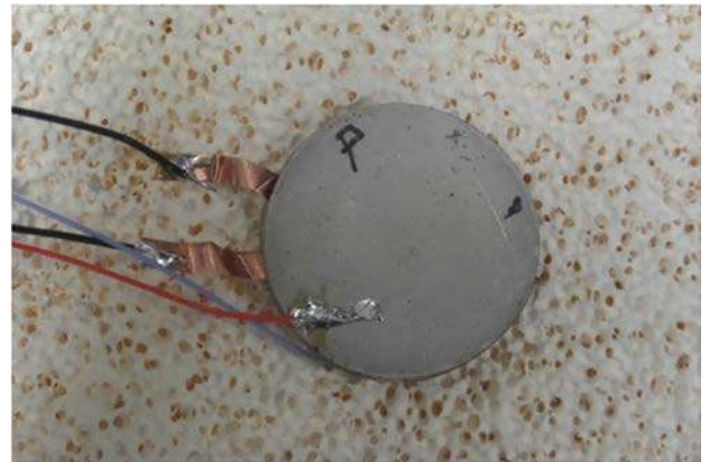
Fig. 3 Prototype of piezoelectric transformer in radial mode
