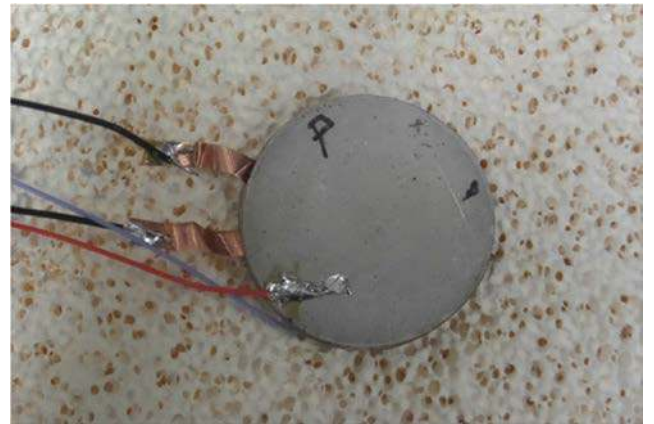
Fig. 3 Prototype of piezoelectric transformer in radial mode
