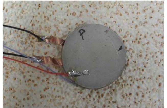
Fig. 3 Prototype of piezoelectric transformer in radial mode
