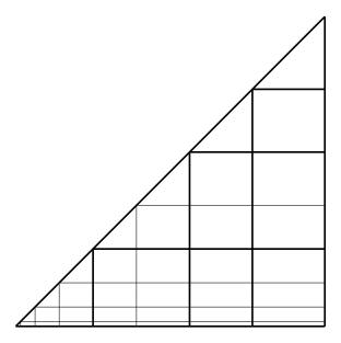
Figure 3: An example of shape-regular quasi-uniform mesh (thicker lines) obtained by patching together elements of the graded mesh (thinner lines).
