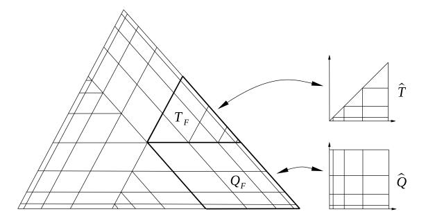
Figure 1: Graded mesh on the triangular face  $F \subset \Gamma$ . The triangular (resp., parallelogram) block of elements  $T_F$  (resp.,  $Q_F$ ) is the image of the graded mesh on the unit triangle  $\widehat{T}$  (resp., the unit square  $\widehat{Q}$ ).
