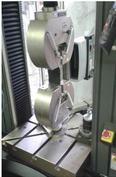
**Figure 7.9: Instron composites tensile testing machine**
