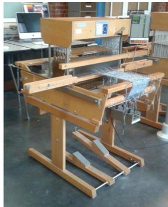
**Figure 7.5: Textile sensors integration during weaving of 2D fabrics, ARM computer controlled hand weaving loom**
