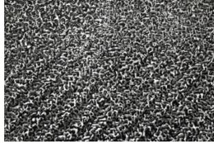
**Figure 5.2: Thermoplastic powdered twill-weave fabric (Chomarat Composites)**
