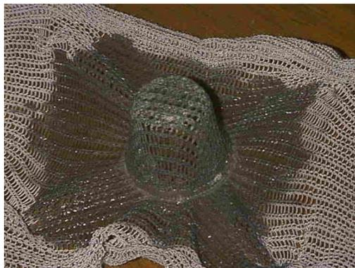
**Figure 3.8: Fabric sample “frozen” with resin**
