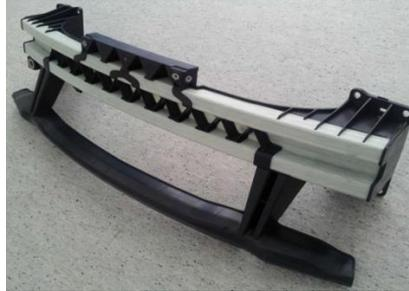
**Figure 5.4: Front bumper crash beam produced with curved reactive thermoplastic pultrusion (Hyundai, Plastic Omnium, CQFD Composites and Arkema)**
