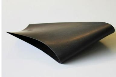
**Figure 5.1: Example of blade manufactured using carbon/epoxy prepregs consolidated in autoclave**
