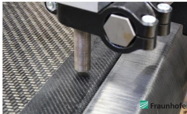
**Figure 6.2: Ultrasonic welding of fibre reinforced thermoplastics**
