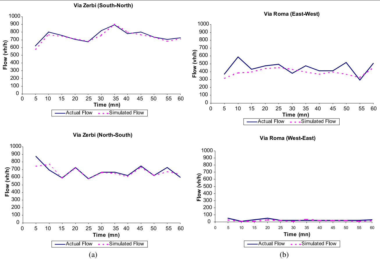
Fig. 17 a Result of the simulation at the Roma–Zerbi intersection in the North–South/South–North directions. b Result of the simulation for the Roma–Zerbi intersection for the East–West/West–East directions
