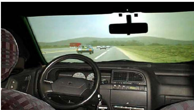
Fig. 1 INRETS Driving simulator and visual environment simulated with ARCHISIM
