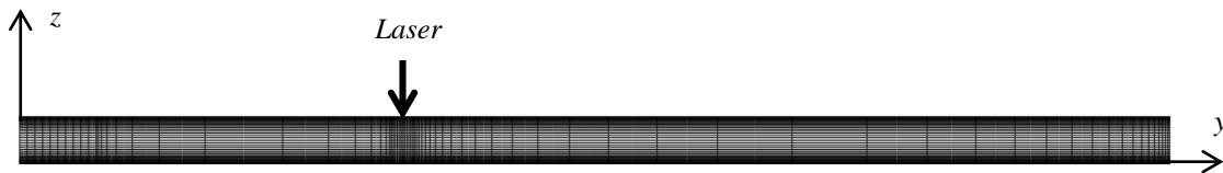
Figure 2 – Finite element mesh of the glass sheet in Figure 1.
