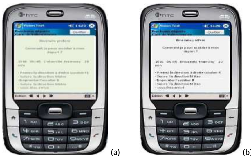
Figure 9. Example of the adaptations of an application to the responsible's speed mobility: normal mobility, normal luminosity (a) and fast mobility, low luminosity (b).
