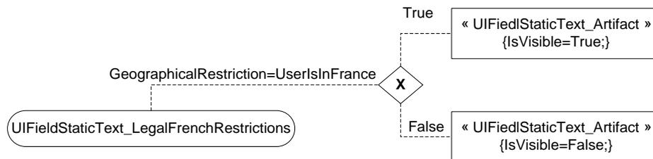
**Figure 8.** Example of use of a geographical restriction in a static interaction model to change the properties associated to the interaction element regarding the geographical localization of the user
