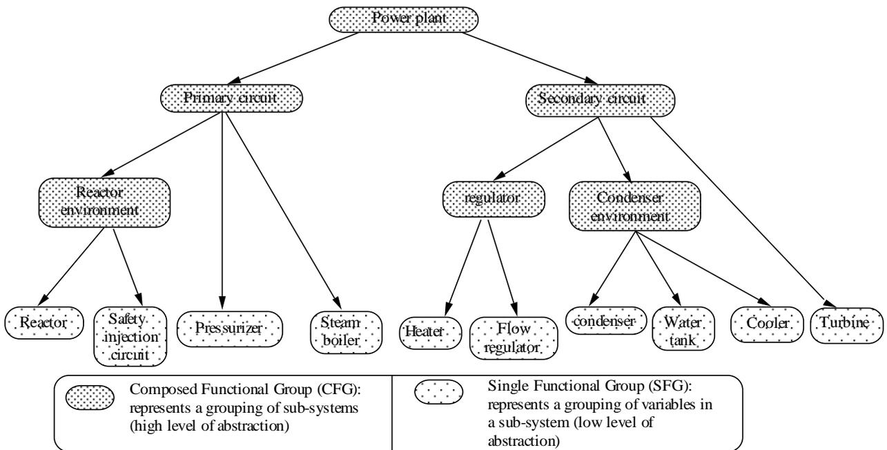
Figure 5. Example of description in three abstraction levels
