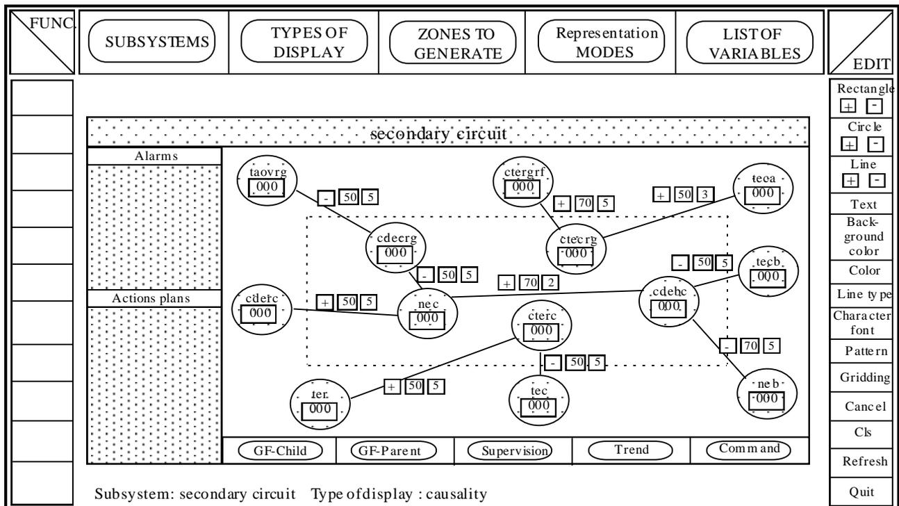
Figure 19. An example of edited display using the "causality network" mode (translated from French)
