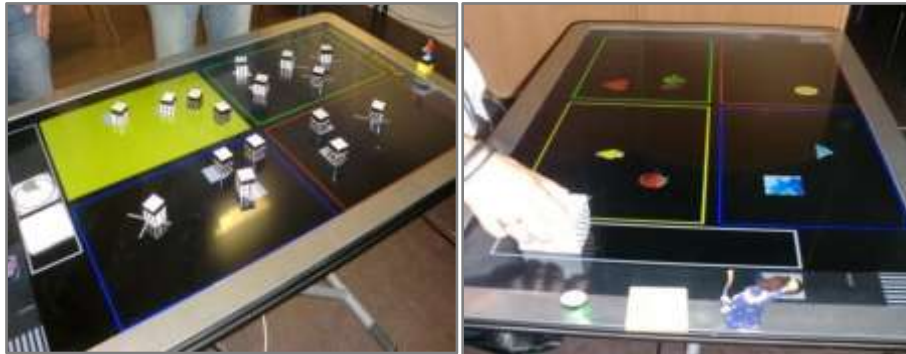
Fig. 1. Two different user interfaces shown on the interactive tabletops with some of used (business and generic) tangible objects: on the left, user Interface displayed on the child tabletop during the correction of exercise; on the right, interface displayed on the adult tabletop during the supervision of the exercise realization
