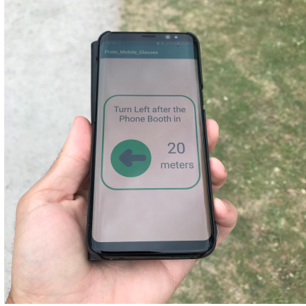
Fig. 1. Mobile Phone Application displaying the instruction: "Turn Left after the Phone Booth in 20 meters"
