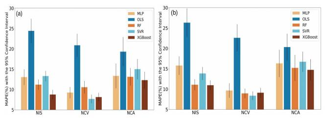
Fig. 5: Mean Absolute Percentage Error (MAPE) for the Nvidia AGX (a) and TX2 (b) GPU platforms with the corresponding 95% Confidence Interval. In this figure we compare the 5 prediction models for exploring: New Image Sizes (NIS), New CNN Variants (NCV) and New CNN Architectures (NCA).
