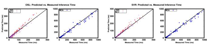
Fig. 6: Predicted vs. Measured Inference Time for OLS (AGX).
