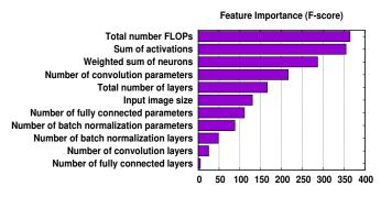
Fig. 3: The feature importance calculated by XGBoost. Features with a high F-score are the most impacting on the CNNs inference time.
