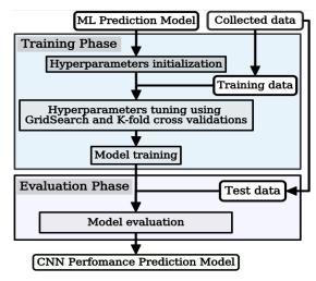
Fig. 4: The process of constructing the prediction models.
