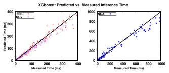
Fig. 15: Predicted vs. Measured Inference Time for XGBoost (TX2).
