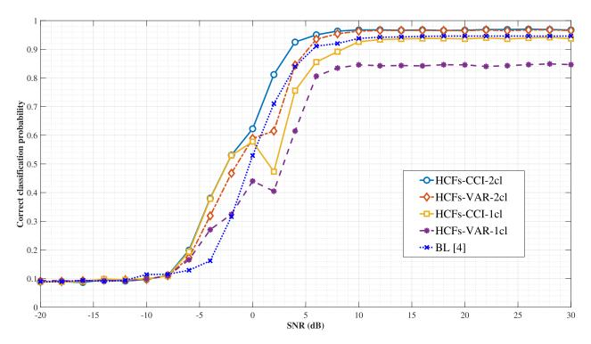
FIGURE 5. Performance comparison of the proposed HCFs selection algorithm, the normalized variance, and the baseline method in [4].
