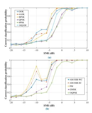
FIGURE 7. Classification performance for individual modulation schemes (a) AM, FM, GMSK, and OQPSK schemes; and (b) OOK, 4ASK, BPSK, QPSK, 8PSK, and 16QAM modulation schemes.
