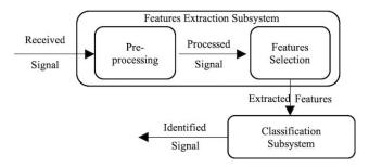
FIGURE 1. Block diagram of the Feature-based AMR method.
