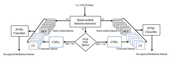
FIGURE 2. Block diagram of the proposed DL-based AMR technique.
