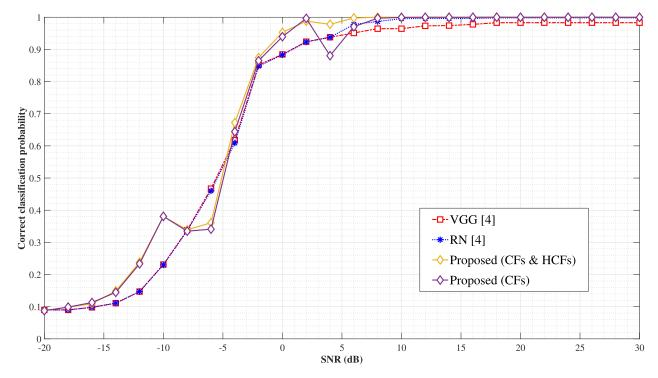
FIGURE 6. Performance comparison of the proposed AMR method.
