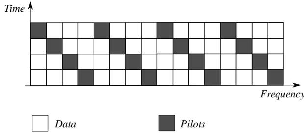
Figure 1. OFDM frame structure with pilot carrier offset.
