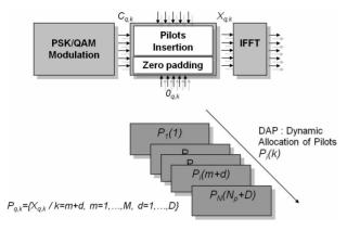
Figure 2. Block diagram of the DAP.
