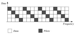
Figure 1. OFDM frame structure with pilot carrier offset.
