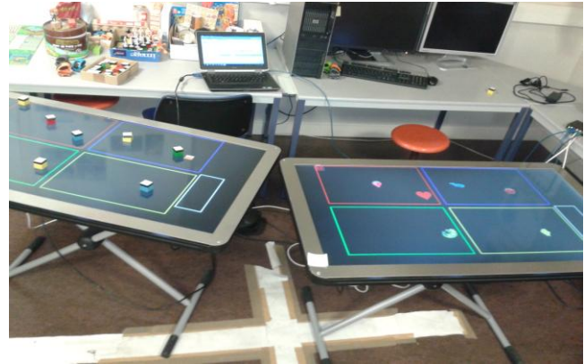
Figure 2. Picture of the distributed application showing the child's view on the left side (with tangible objects) and the parents' view on the right side (with virtual objects as feedback).
