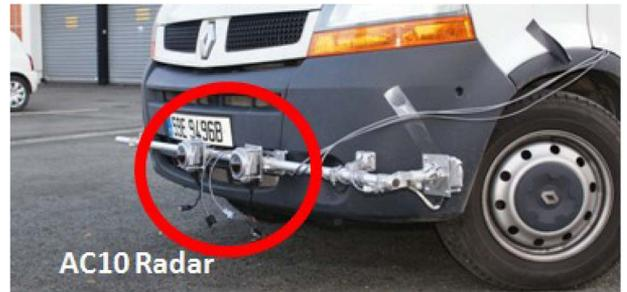
Fig. 2. Car with AC10 radar.
