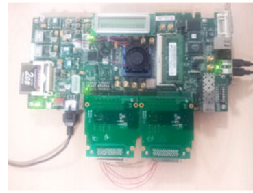
Fig. 14. ML605 kit showing FMC connector loopback using MIL-STD-1553.
