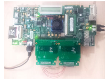
Fig. 14. ML605 kit showing FMC connector loopback using MIL-STD-1553.
