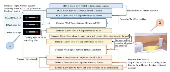
Fig. 2. Model of cooperation between Human, BCI and Robot according to their Know-How and their Know-How-to-Cooperate, Common Work Space between BCI and Human (1), Common Work Space between Human and Robot (2)
