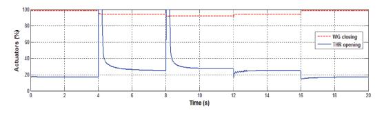
**Figure 3.** Pressure tracking performance (up) and corresponding actuator commands (bottom) with conventional MIMO controller at  $N_e = 2000$  rpm.
