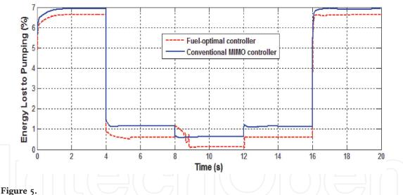
Comparison of engine pumping losses between conventional MIMO controller and fuel-optimal controller at  $N_e = 2000$  rpm.
