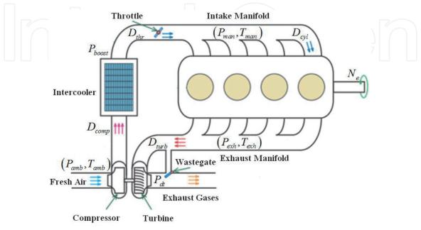
**Figure 1.** Schematic of a turbocharged spark-ignition engine.
