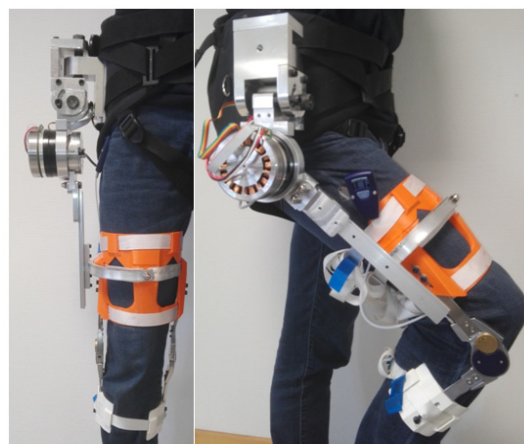
Figure 2: First prototype - Hip only actuated exoskeleton.
