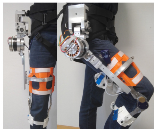
Figure 2: First prototype - Hip only actuated exoskeleton.
