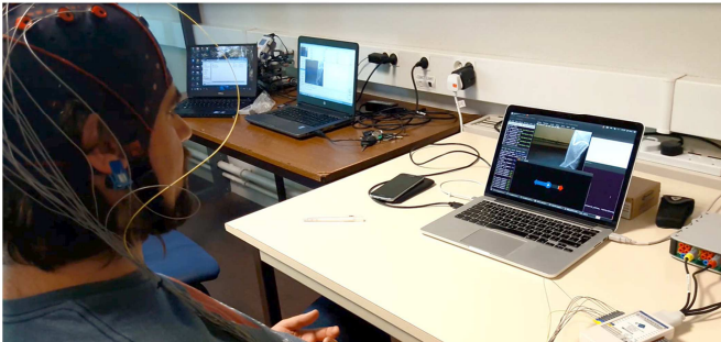
Fig. 7. BCI/Emulated haptic control interface. Visual feedback is provided about the state of the BCI system as well as the environment in which the robot is operating.
