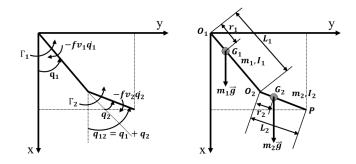
Fig. 1. Description of a 2-DoF robot.
