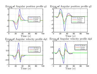
Fig. 5. Tracking errors of angular position and velocity profile.
