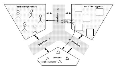
Fig. 2: Human and artificial agents acting on the process<sup>1</sup>.
