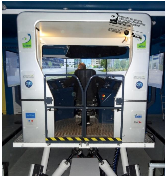
Figure 11. The rail simulator of the University Polytechnique Hauts-de-France.
