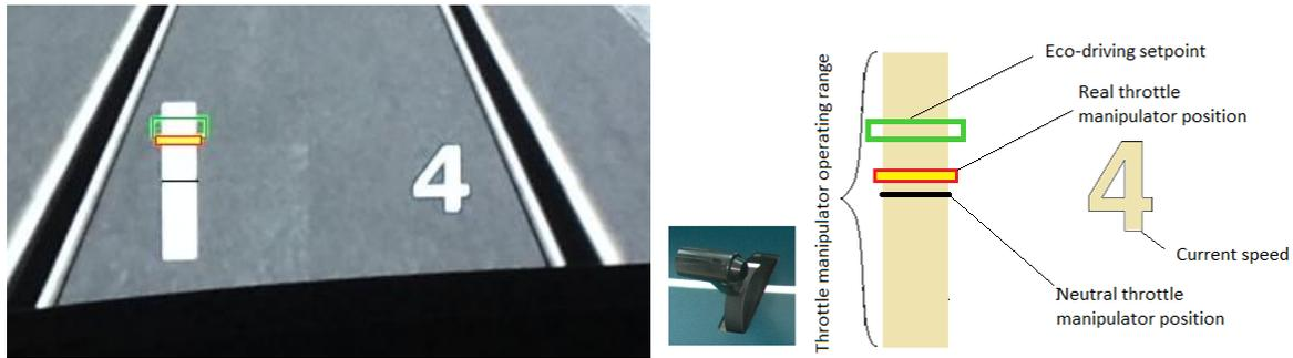
Figure 10. Human-Machine Interface in Head-Up Display (HUD).
