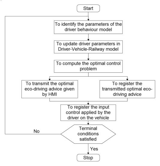
Figure 7. The recursive CEDRICS algorithm principle.
