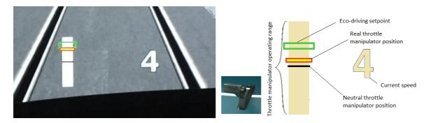
Figure 10. Human-Machine Interface in Head-Up Display (HUD).
