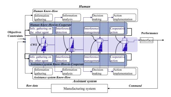
Figure 1. Human-machine cooperation model from (Pacaux and al. 2017).
