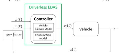
Figure 3. Driverless EDAS configuration.
