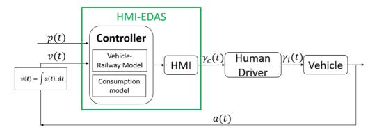
Figure 4. HMI-EDAS configuration.
