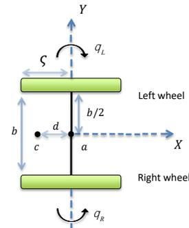
Figure 3. Simplified top view of the wheelchair
