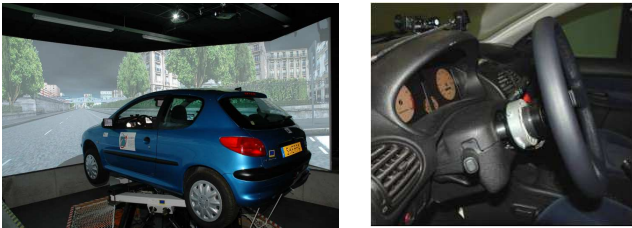
Fig. 9. SHERPA driving simulator (left), steering torque sensor (right).
