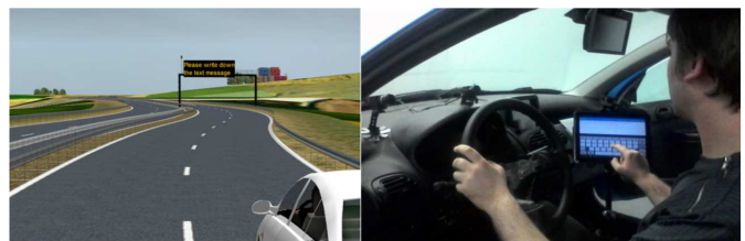
Fig. 19. The variable road sign inviting the driver to write the text message (left); the driver performing the secondary task (right).
