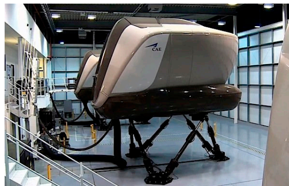
Figure 5. Integrated CAE 7000XR flight simulator [12].
