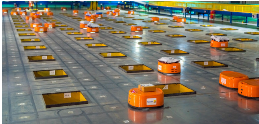
Figure 1. A material handling system for e-commerce product sortation (Indian Flipkart [7]).
