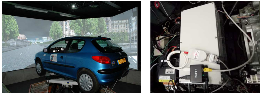
Figure 6: SHERPA interactive dynamic driving simulator (left). Data acquisition system (right).
