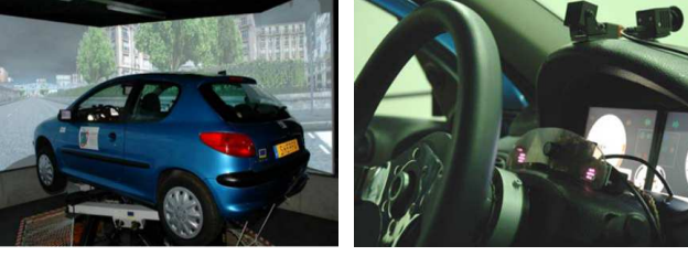
Fig. 8. SHERPA driving simulator (left); steering torque sensor and Continental driver monitoring system (right).
