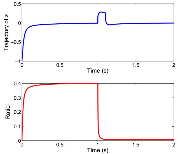
**Fig. 2** Trajectory of the performance output  $z$  and the ratio  $\frac{\int_0^\infty z(t)^\top z(t) dt}{\left(\int_0^\infty w(t)^\top w(t) dt + \rho\right)}$  corresponding to the results presented in Fig. 1.
