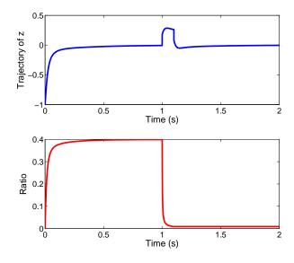
Fig. 2 Trajectory of the performance output z and the ratio  $\int_{0}^{\infty} z(t)^{\top} z(t) dt / \left( \int_{0}^{\infty} w(t)^{\top} w(t) dt + \rho \right)$  corresponding to the results presented in Fig. 1.
