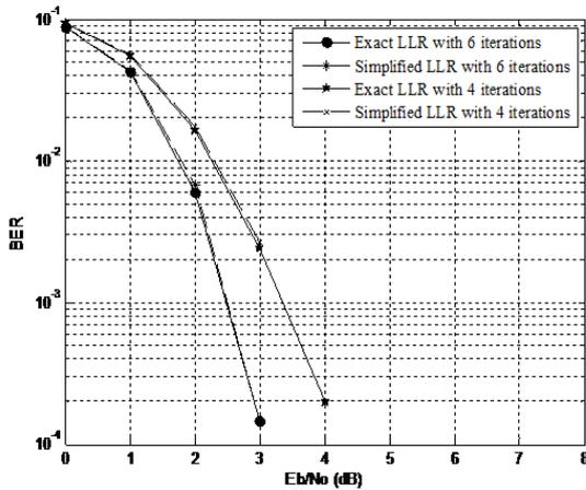
Fig. 2. Performance comparisons, under Gaussian channel, of (512, 1024) LDPC code using exact and simplified LLR algorithms, with 4 and 6 iterations (frame =20)
