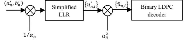
Fig. 1. Principle of simplified LLR calculation
