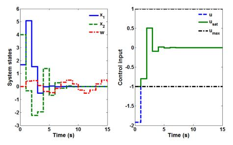
Figure 6: Case 2 with  $\beta_2^* = 1.68$ . Closed-loop behaviors of T-S system (61) corresponding to the initial condition  $x_0^{\top} = [\beta_2^* \ 4]$  obtained for the non-PDC controller with matrices given in (65).
