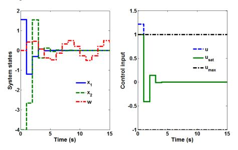
Figure 4: Case 1 with  $\beta_1^* = 1.55$ . Closed-loop behaviors of (61) corresponding to the initial condition  $x_0^{\top} = [\beta_1^* - 4]$  obtained for the non-PDC controller with matrices given in (64).
