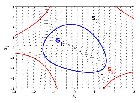
Figure 3: Results obtained with  $\beta = 1.6$ : guaranteed domain of attraction  $S_1 = \mathcal{E}_{\mathbb{V}}$ , generalized sector condition for input saturation  $S_2 = \mathcal{P}_u$ , domain of validity  $S_3 = \mathcal{P}_x$ .
