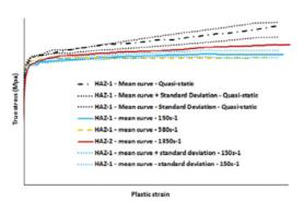
**Figure 10.** HAZ – True stress-strain curve – Strain rate dependency.
