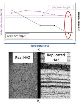
**Figure 2.** a) Description of the optimized heat treatment; b) comparison of real and replicated HAZ microstructure.
