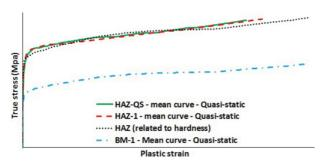
Figure 7. BM and HAZ quasi-static true stress-strain curves.
