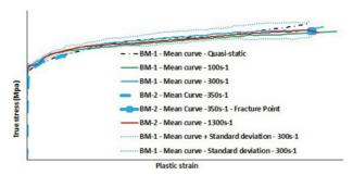
Figure 8. BM – True stress-strain curve – Strain rate dependency.
