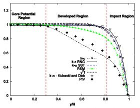
Fig. 5. Comparison of dimensionless wall-normal velocity obtained by five turbulence models at jet center line with k- $\omega$  [7] and PIV data
