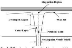
Fig. 1. Different region of a confined impingement jet flow
