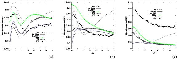
Fig. 11. Non-dimensional Turbulent Kinetic Energy (TKE) across horizontal lines in impact region. (a) y/e=9, (b) y/e=9.5 and (c) y/e=9.8.
