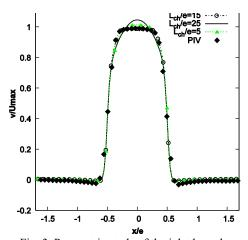
Fig. 3. Parametric study of the inlet boundary condition at the nozzles exit compared against PIV results
