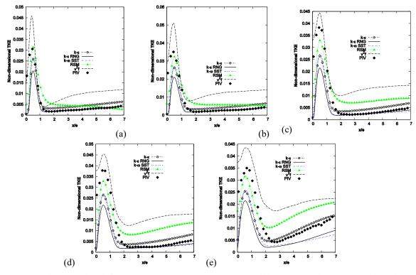
Fig. 9. Non-dimensional Turbulent Kinetic Energy (TKE) across horizontal lines in developing region. (a) y/e=4, (b) y/e=5, (c) y/e=6, (d) y/e=7 and (e) y/e=8.
