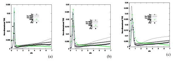
Fig. 7. Non-dimensional Turbulent Kinetic Energy (TKE) across horizontal lines in potential core region. (a) y/e=1, (b) y/e=2 and (c) y/e=3.
