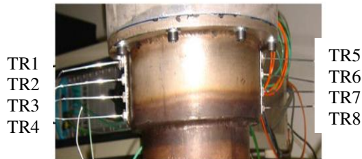
FIGURE 2. REGENERATOR INSTRUMENTATION ( 8 THERMOCOUPLES ARE POSITIONED IN THE REGENERATOR)
