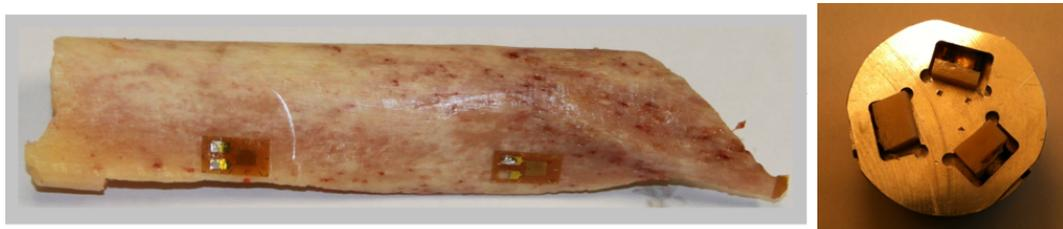
Figure 4: Bone specimens holder for polishing stage and nanoindentation experiments
